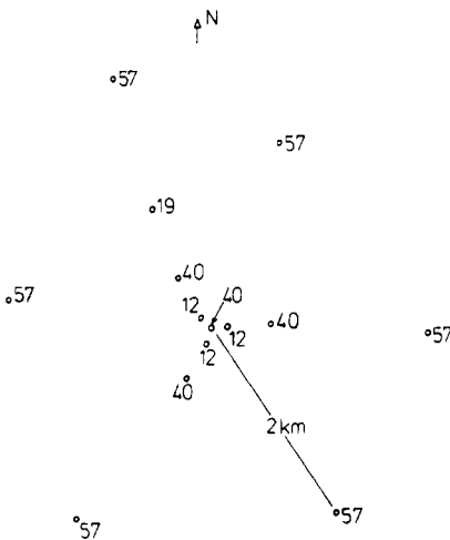
Figure 1. The detector arrangement at the Haverah Park EAS array. The number at each detector corresponds to the volume of water-Čerenkov detector (in \text{m}^3 ) at that point.
